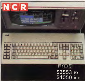
NCR PC4i - 256KB RAM, Colour or mono, dual floppies or 10MB. Fully IBM compatible. NCR field service Australia wide.
